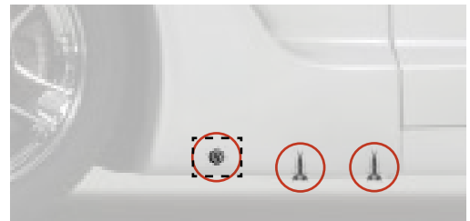
Three screws need to be removed; two vertical and one horizontal.
