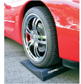
Flatspotting happens when a tire is compressed against a hard surface while the car is parked. A section of the rubber becomes softer or stiffer than the rest of the tire. The tire flat spots cause a noticeable disturbance when the car is in motion. Flat spotted tires can cause vibrations as soon as you pull out of the garage, but sometimes are only noticeable at higher speeds when you get out on the highway.
