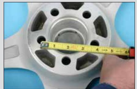
I measured a five-bolt wheel's bolt circle by measuring from the center of one hole to the outer edge of a hole furthest away from the first hole. In this example, we see a measurement that's just under 4 inches. However, it can be difficult for a novice to accurately place a tape measure or ruler at the exact center of the first hole. In this case, the circle is minutely less than 4 inches (it's actually a 100mm circle or 3.9937 inches).
