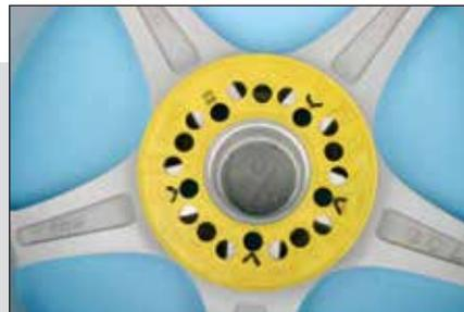
In this example, I used a bolt circle template. Once I find a series of five holes that align with the holes in the wheel, I'll note that this wheel does indeed feature a 100mm bolt circle.
