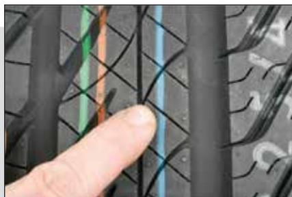
The smallest cuts in tread blocks are referred to as sipes. They provide added traction on wet or icy surfaces.
