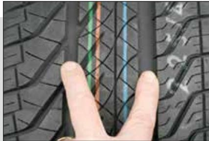
Longitudinal grooves in the tread allow for immediate water passage.
