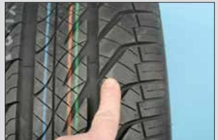
Angled grooves, referred to as lateral grooves, direct water out from the longitudinal grooves to aid in water evacuation. Water is collected in the main grooves and directed out of the tread area via lateral grooves.
