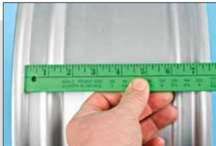
Rim width is measured between the bead walls, not at the overall width. This wheel measures 7 inches between the bead walls.
