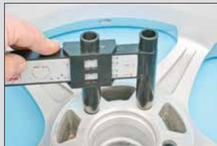
The bolt circle caliper gauge in use. When using this specific tool, measure two bolt holes that are immediately adjacent to each other (the tool has been calibrated to use these locations). Insert carefully and allow the gauge to slide while the tapered dowels find true center. Always insert from the hub face since the holes at the front of the wheel will typically be too far recessed to use this tool.
