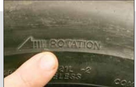
Directional tires will feature a mark on the sidewall indicating direction of rotation. You won't damage the tire if mounted backward but you'll greatly diminish the performance advantages that the tire offers.
